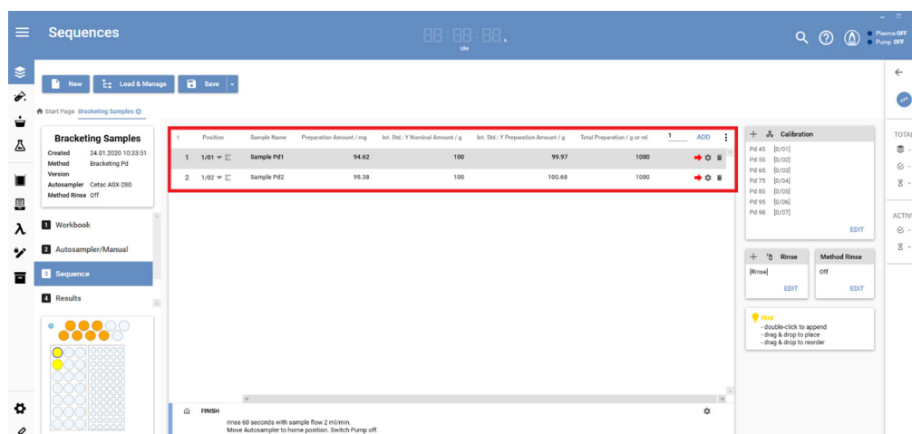
Figure 7: Sequence view of the ICP Analyzer Pro software with a bracketing setup
