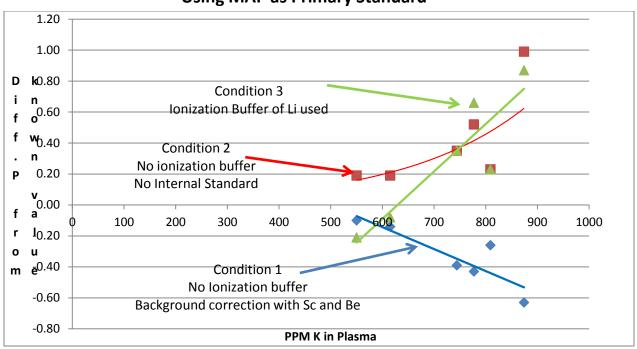
ICP for Phosphate Using Different Conditions Using MAP as Primary Standard
